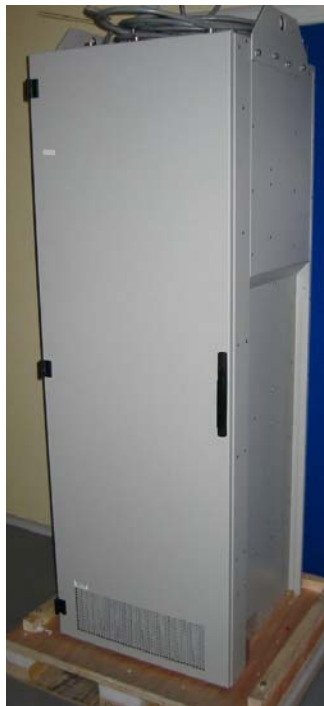
Figure 2: GSM 18000 Indoor NG2 BTS Front side.
