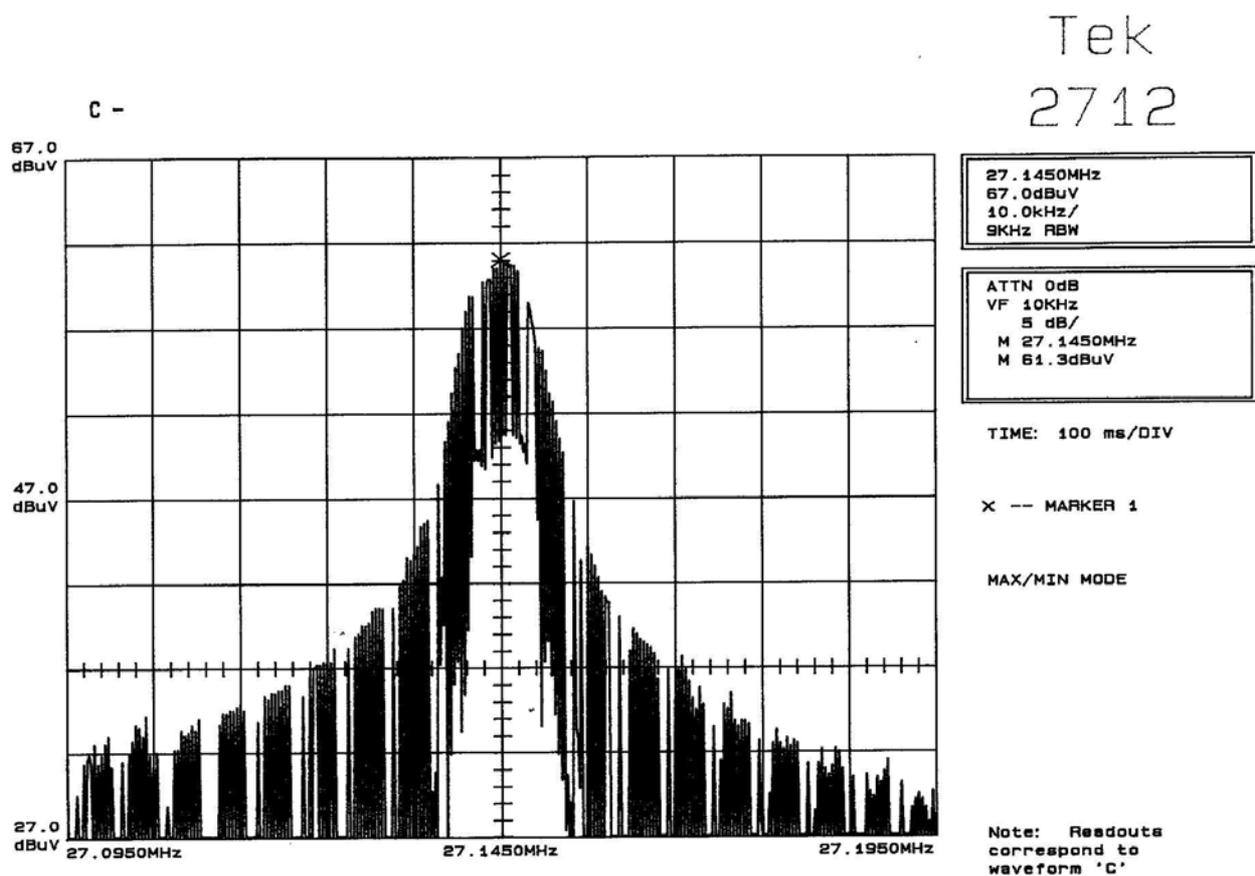
Result : The field strength of any emission within the operation band did not exceed 80 dB( $\mu$ V/m) for average value or 100 dB( $\mu$ V/m) for peak value. Refer to page 9 for the recorded value for the emission at the fundamental frequency.
