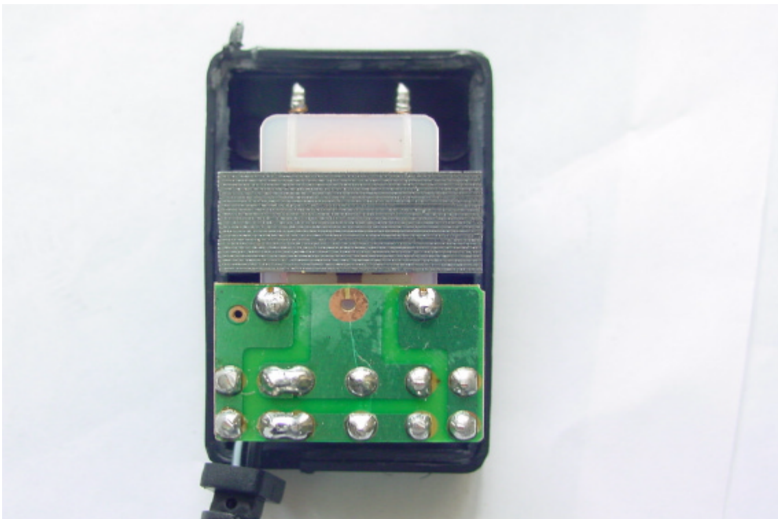
Solder View of Adaptor's PCB
