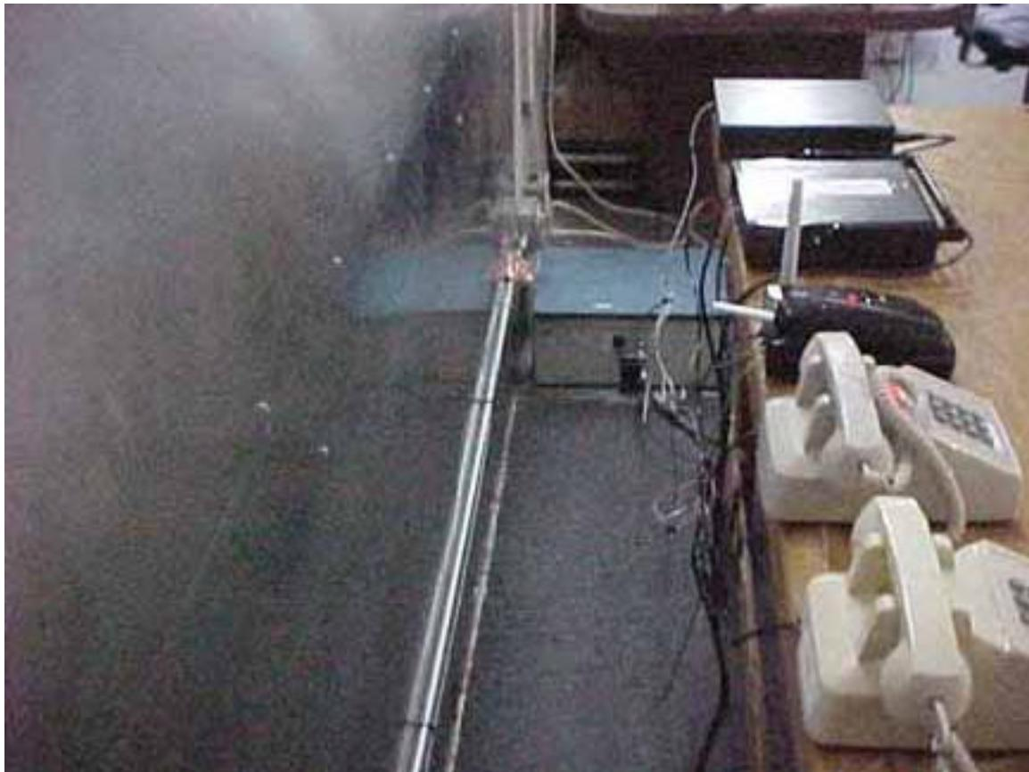
**REAR VIEW****2.4 GHz / 900 MHz CORDLESS PHONE - BASE****MODEL: CP-2575****FCC SUBPART B and C - CONDUCTED EMISSIONS – 3-10-00****PHOTOGRAPH SHOWING THE EUT CONFIGURATION
