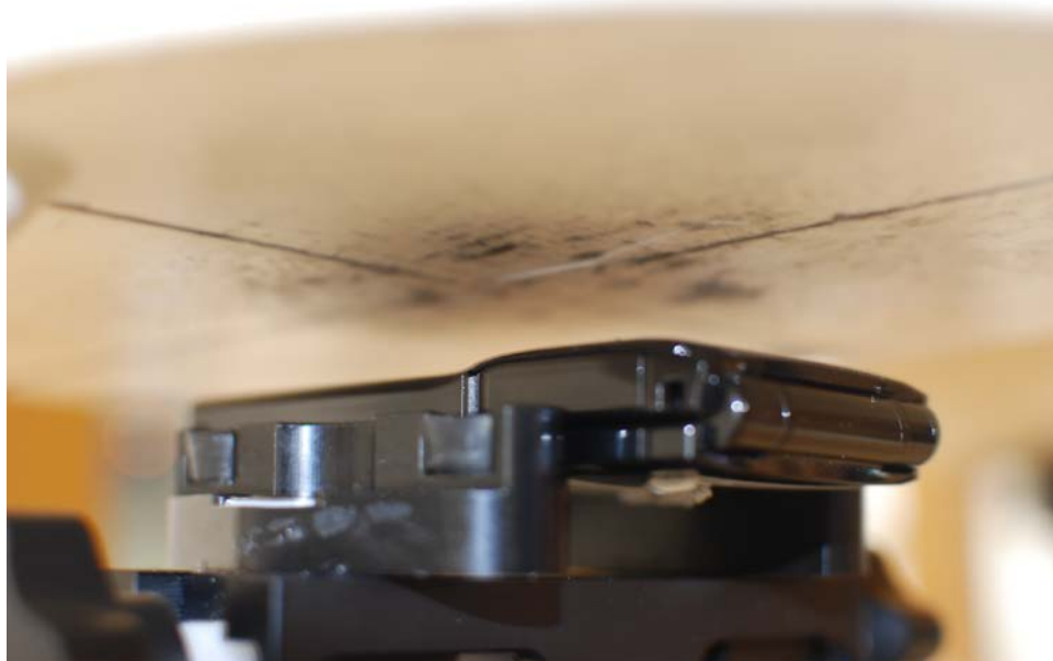
SAR Test Setup Photo 6: Body-Worn at 15mm
