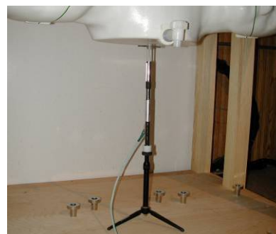
Figure 12-2 System Verification Setup Photo
