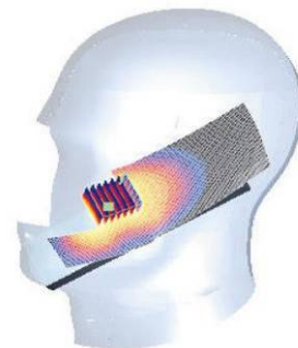
Figure 7-1 Sample SAR Area Scan
