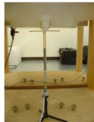
900MHz System performance check setup
