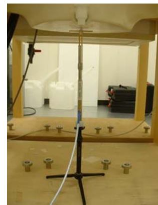
1800MHz System performance check setup
