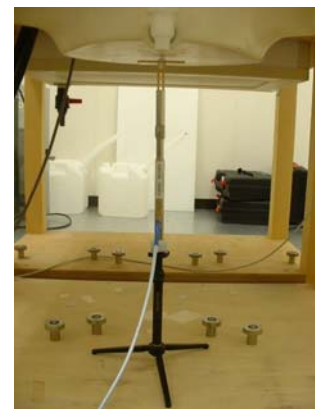
1800MHz System performance check setup
