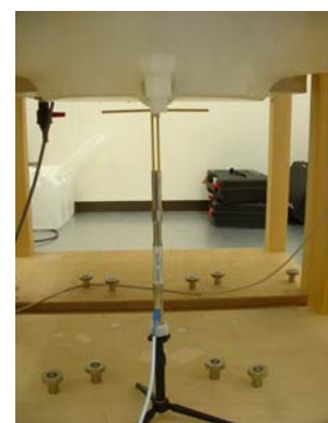
900MHz System performance check setup
