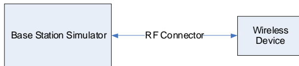
Figure 13-1 Power Measurement Setup
