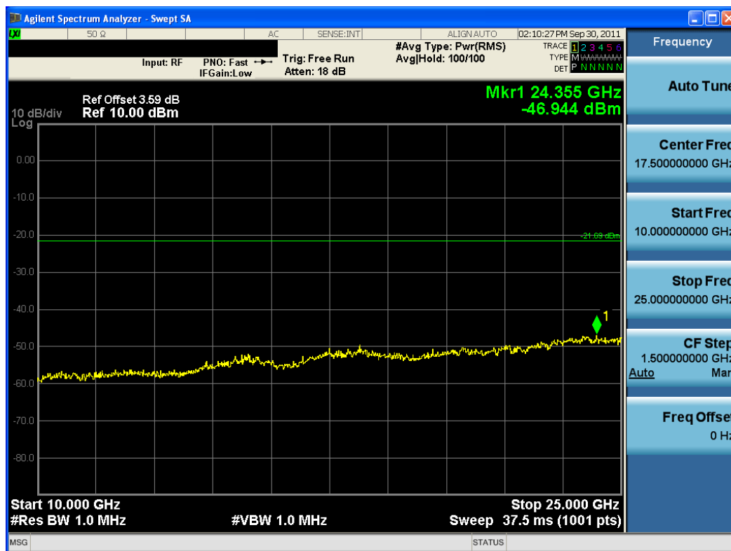
Plot 6-14. Conducted Spurious Plot (Bluetooth (LE) – Ch. 39)
