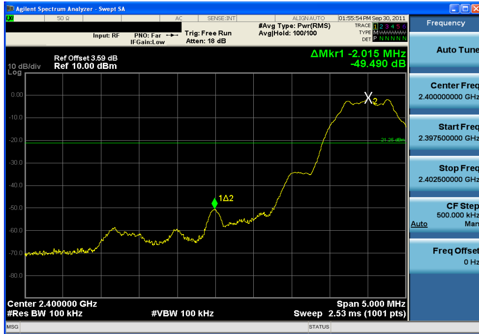
Plot 6-7. Band Edge Plot (Bluetooth (LE) – Ch. 0)
