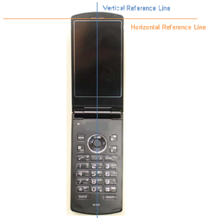
SAR Test Setup Photo 7: Horizontal and Vertical Reference Lines
