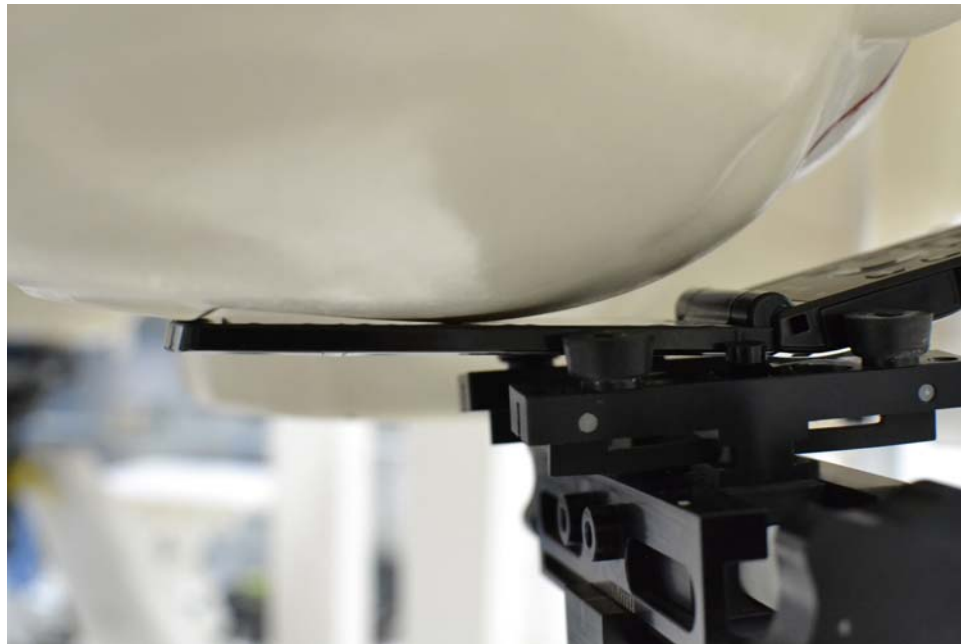
SAR Test Setup Photo 2: Right Cheek
