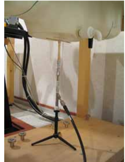
Photo of the dipole Antenna
