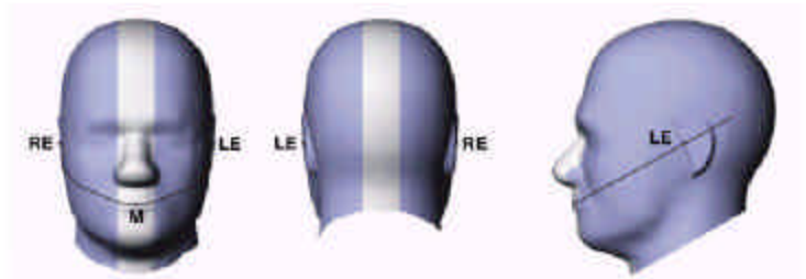
Figure 9-2 Front, back and side view of SAM Twin Phantom
