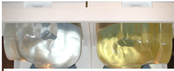
Figure 7.1 Left and Right SAM Phantom shells
