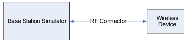
Figure 13-1 Power Measurement Setup
