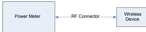
Figure 12-1 Power Measurement Setup
