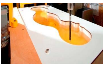
Figure 6-2 SAM Phantom with Simulating Tissue
