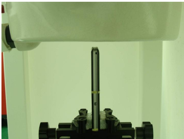
Bottom Side with Phantom 1 cm Gap
