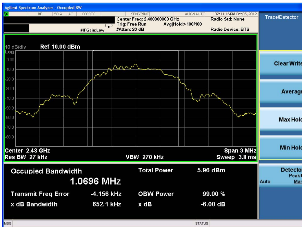
Plot 6-3. 6dB Bandwidth Plot (Bluetooth (LE) – Ch. 39)
