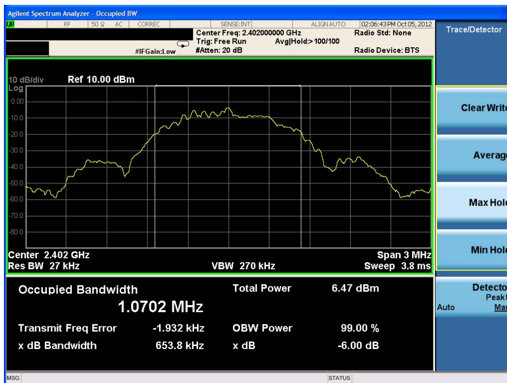
Plot 6-1. 6dB Bandwidth Plot (Bluetooth (LE) – Ch. 0)
