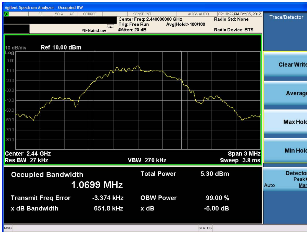
Plot 6-2. 6dB Bandwidth Plot (Bluetooth (LE) – Ch. 19)
