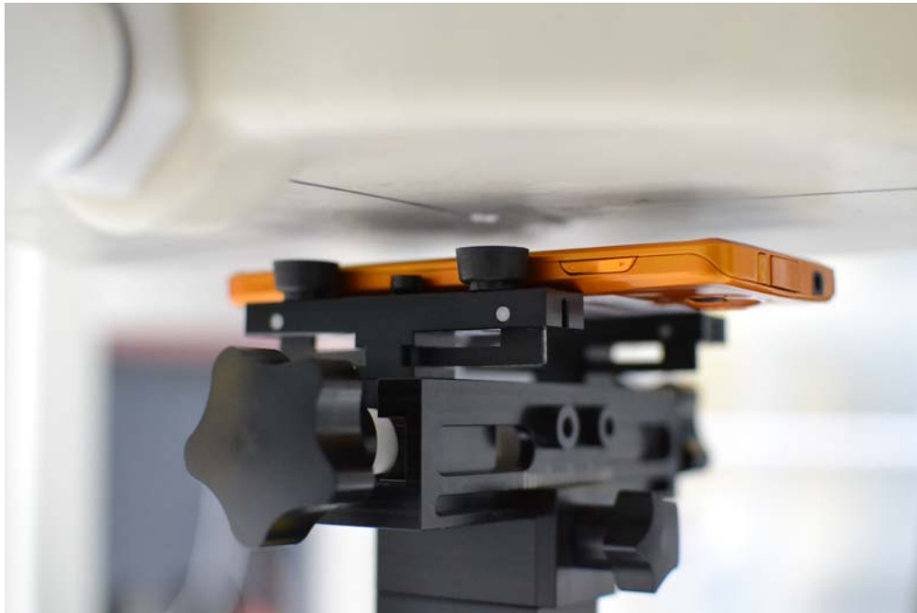
SAR Test Setup 6 - Front Side at 1.0 cm
