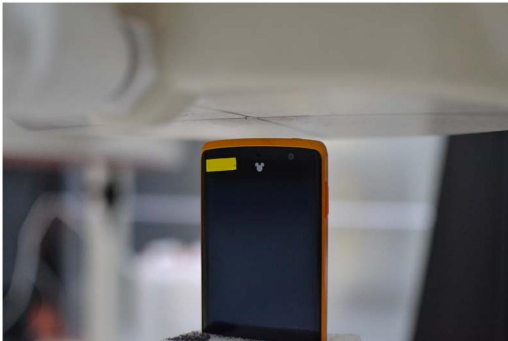
SAR Test Setup 8 - Top Edge at 1.0 cm
