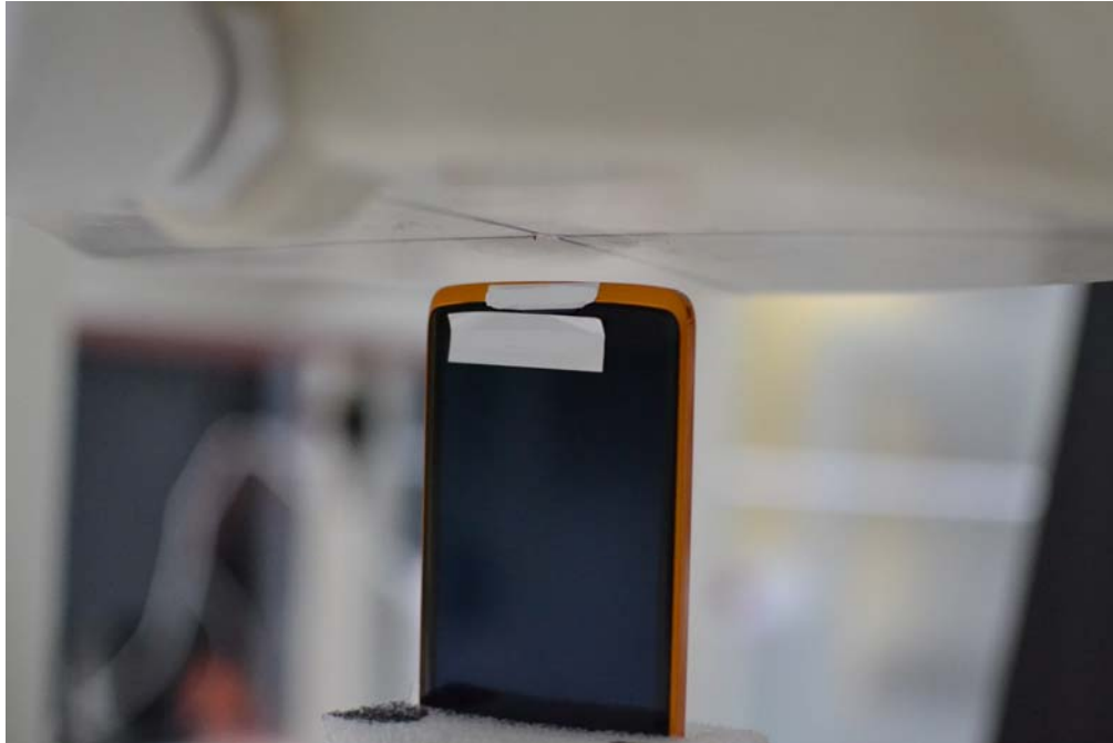
SAR Test Setup 7 - Bottom Edge at 1.0 cm
