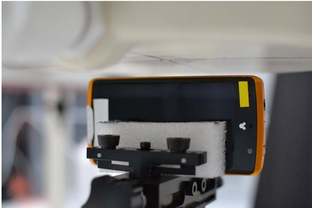
SAR Test Setup 10 - Left Edge at 1.0 cm
