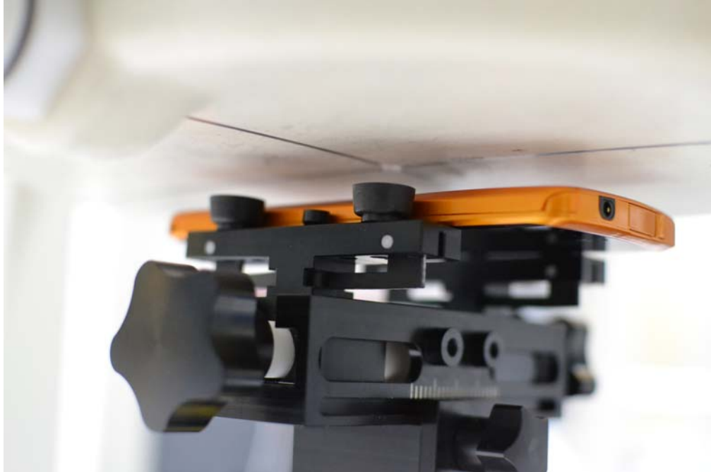
SAR Test Setup 5 - Back Side at 1.0 cm
