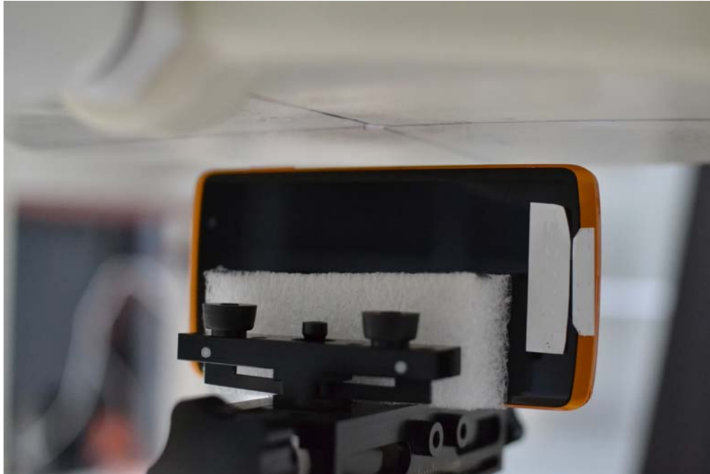
SAR Test Setup 9 - Right Edge at 1.0 cm
