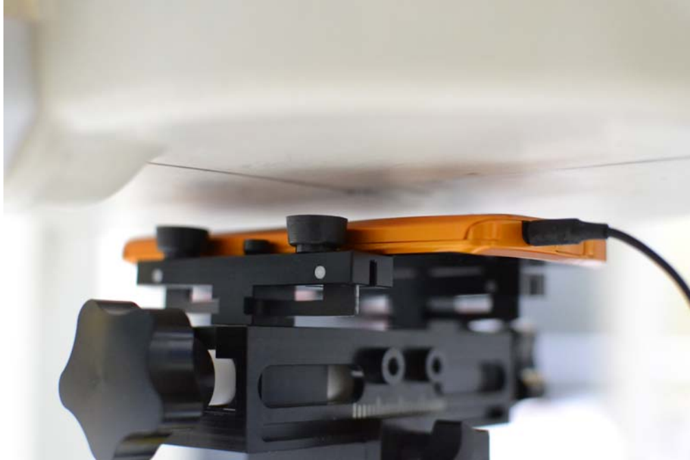
SAR Test Setup 11 - Body-Worn Back Side at 1.0 cm
