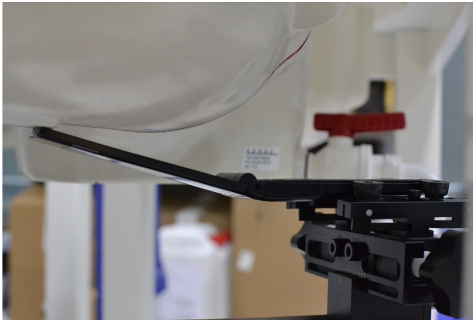
SAR Test Setup Photo 2 – Right Tilt
