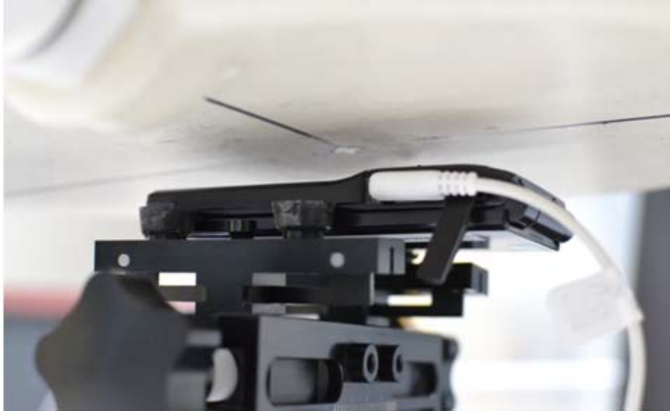
SAR Test Setup Photo 5 – Body Worn Back Side 1.5 cm
