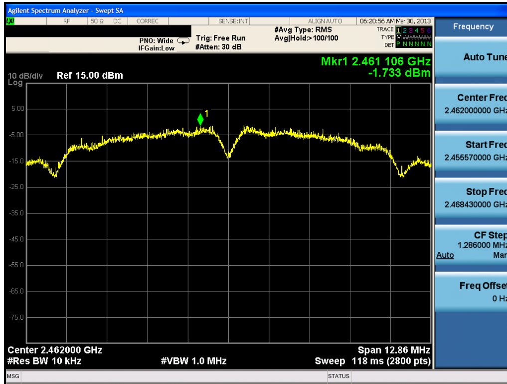
Plot 6-15. Power Spectral Density Plot (802.11b – Ch. 11)
