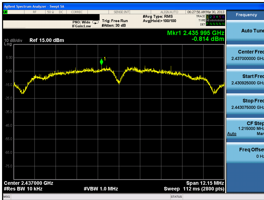
Plot 6-14. Power Spectral Density Plot (802.11b – Ch. 6)
