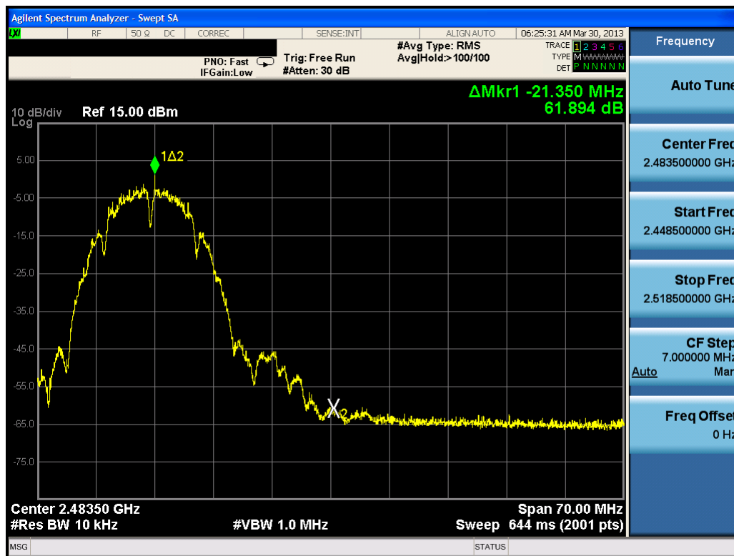
Plot 6-26. Band Edge Plot (802.11b – Ch. 11)
