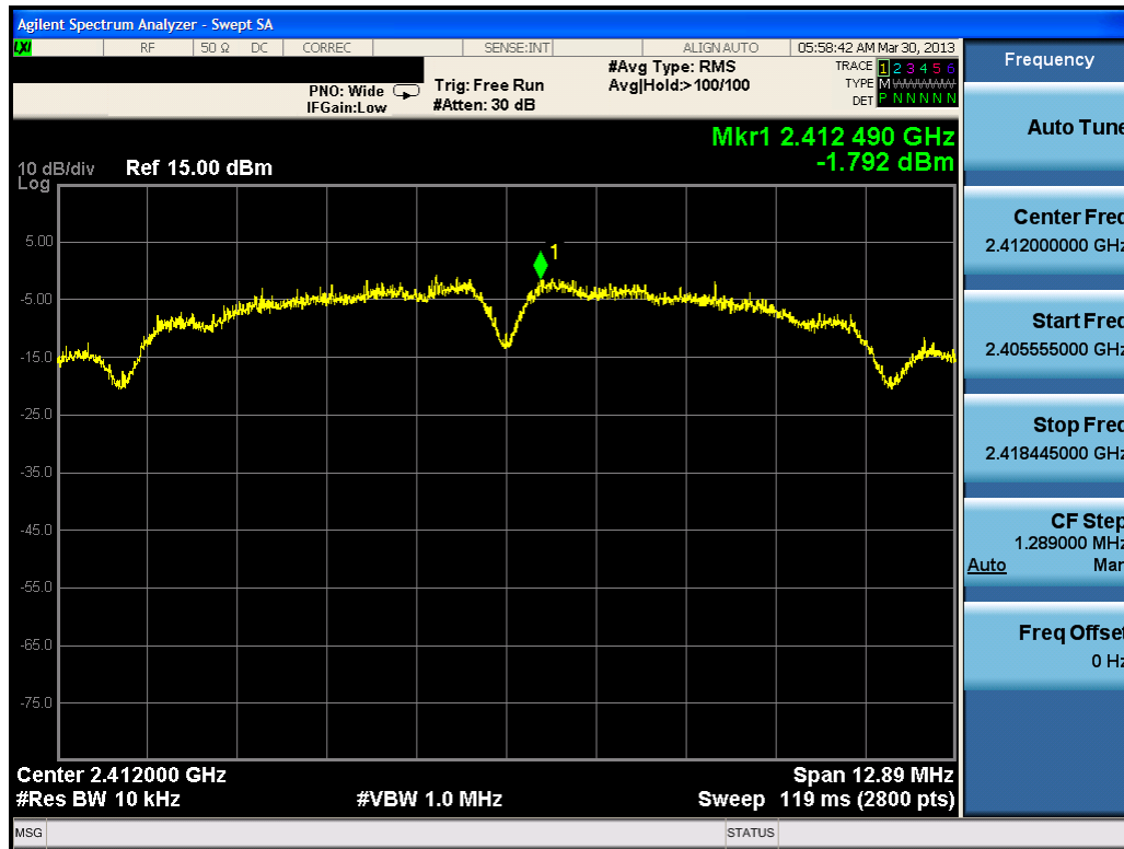
Plot 6-13. Power Spectral Density Plot (802.11b – Ch. 1)
