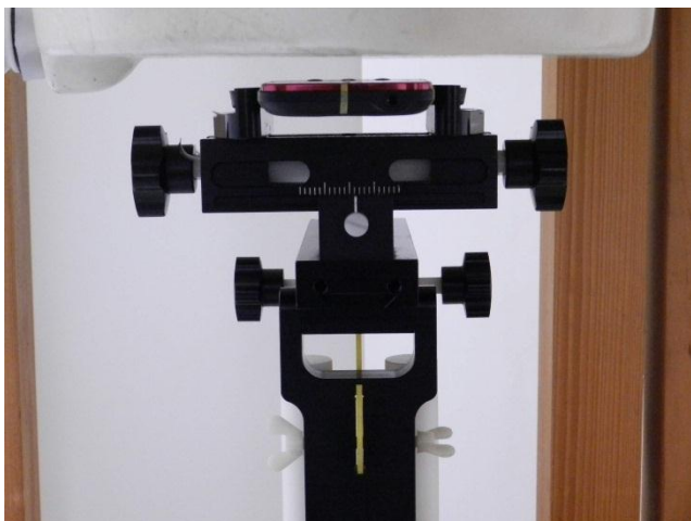
Front of the DUT with Phantom 1 cm Gap (without Headset)
