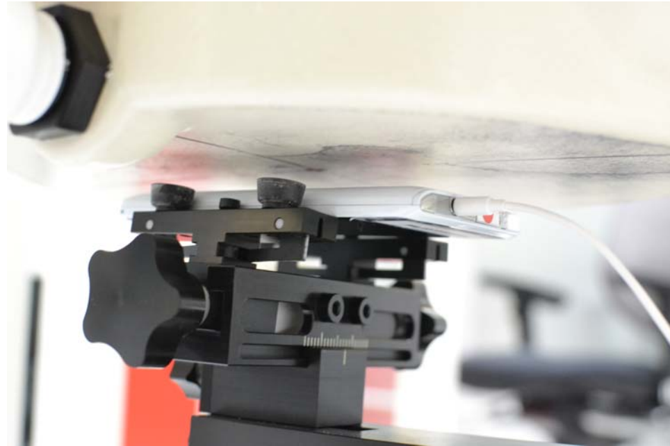
SAR Test Setup Photo 11: Back Side Body-Worn at 1.0 cm
