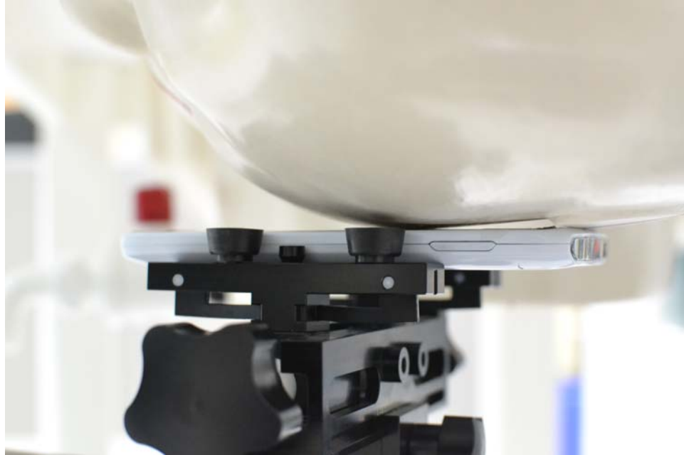
SAR Test Setup Photo 3: Left Cheek
