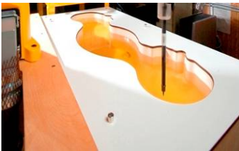
Figure 6-2 SAM Phantom with Simulating Tissue
