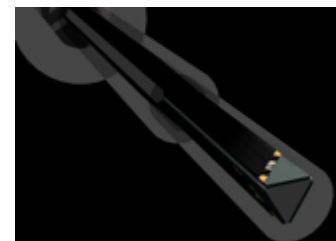
Figure 5-3 Triangular Probe Configuration
