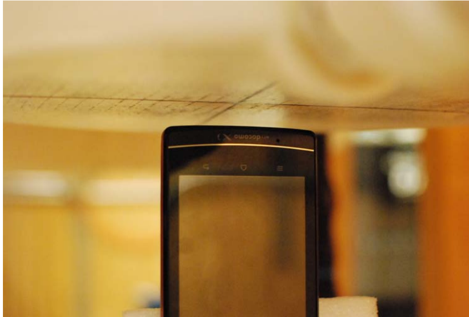
SAR Test Setup Photo 7: Bottom at 1.0 cm
