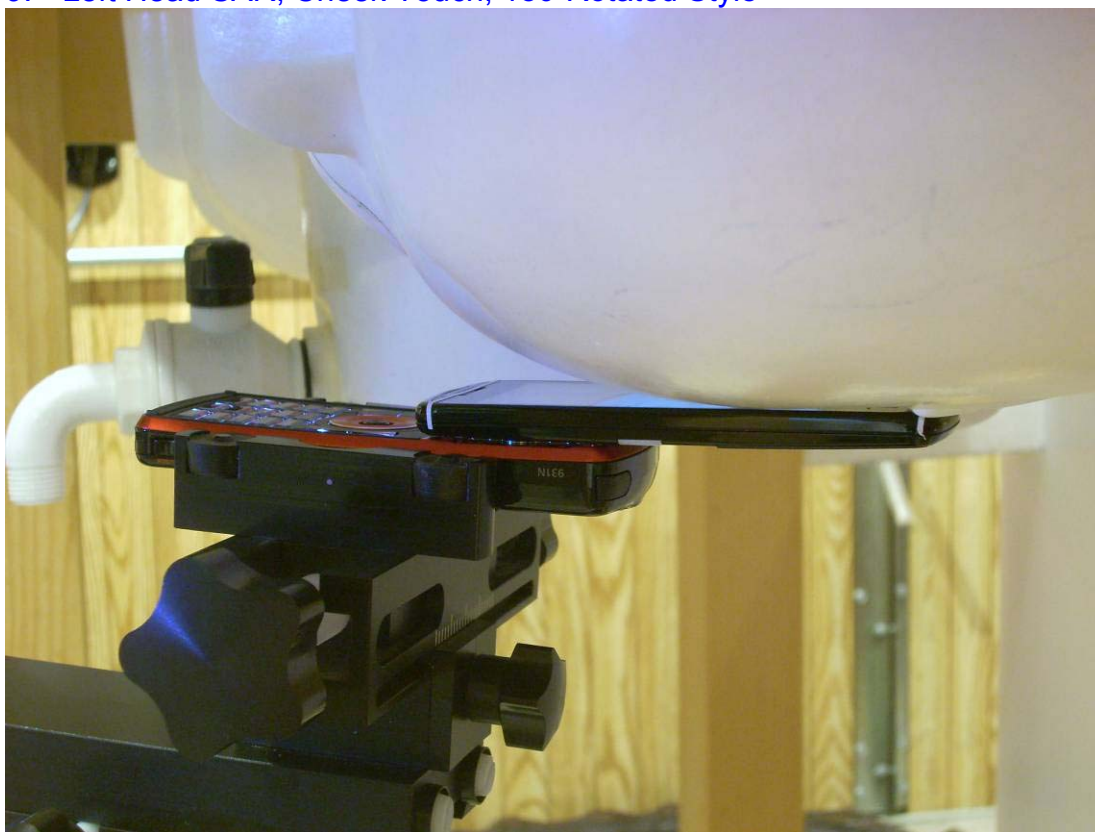
10. Left Head SAR, 15° Tilt, Slide Out, 180-Rotated Style
