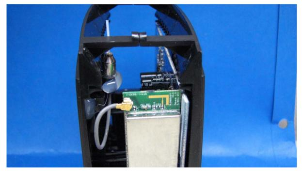
Change in Radio module can grounding:
