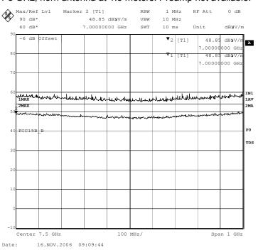
c. 7-8 GHz, 4-8 GHz, horn antenna at 1.5 meters. Preamp not available.
