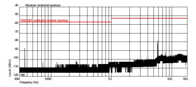
Conclusion: The maximum receiver conducted spurious at the antenna port is -79 dBm, or 0.0125 nW.
