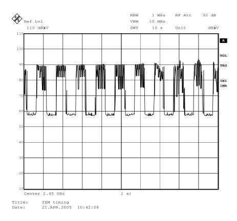
2: Time scale 1 msec/division, trace triggered on the RF signal "on" time = 501usec repetition time 7.47 ms duty cycle 6.8%
