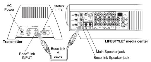
Note: If another product is already connected to the Bose link Speaker jack on the media center, disconnect it there. You can use the wireless audio link to replace that wired connection. Or, to continue using that connection, reconnect the cable to the jack labeled Bose link OUTPUT on the transmitter connection panel (Figure 4).
