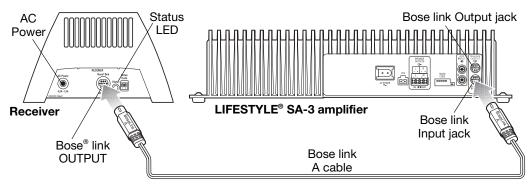
3. Insert the small plug on the power pack cable into the AC Power jack on the receiver and plug the pack into a wall outlet.
