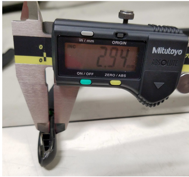
Measured Distance from the inner surface of the antenna to the body side of the enclosure
