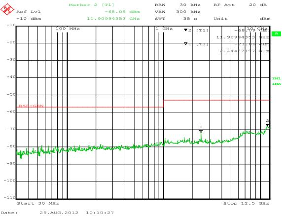
Measurements from 30MHz - 12.5 GHz, RX mode, and receiver tuned to mid-band. Highest reading of -68.09dBm or 0.155nW was measured at 11.91 GHz, this passes by 15.0 dB
