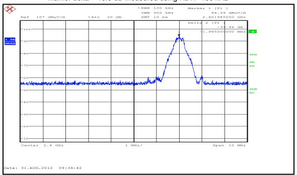
Marker delta = 40.0 dB measured using RBW=100 kHz
