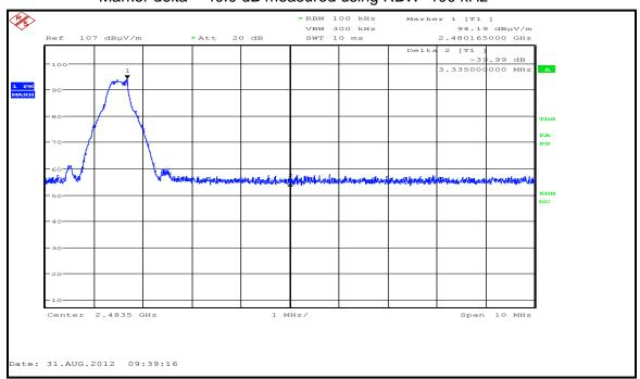
Marker delta = 40.0 dB measured using RBW=100 kHz
