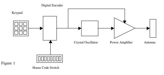
Y1: Crystal oscillator 27.145 MHz (Transmitter) Y2: Clock generator 4.0 MHz (Micro processor)
