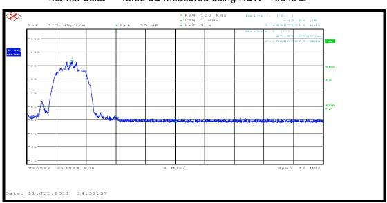
Marker delta = 43.66 dB measured using RBW=100 kHz
