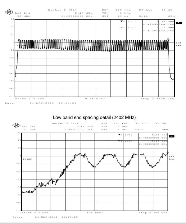
79 channels between 2402 MHz and 2480 MHz = 1 MHz/channel
