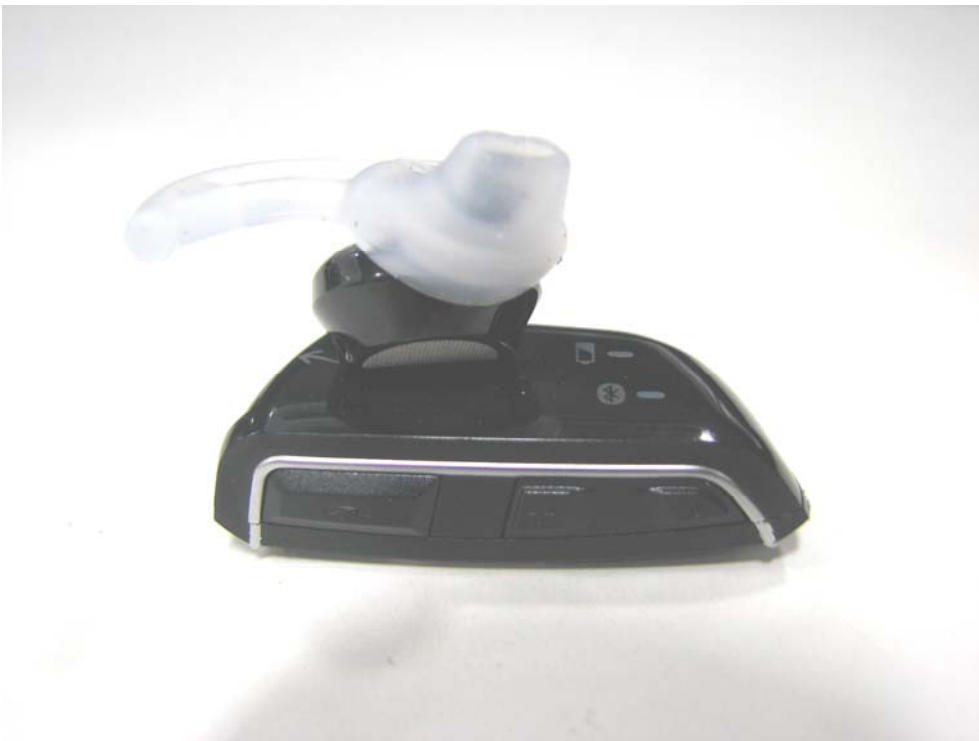
Close up picture of Bluetooth earpiece – side view showing volume and answer/end buttons
