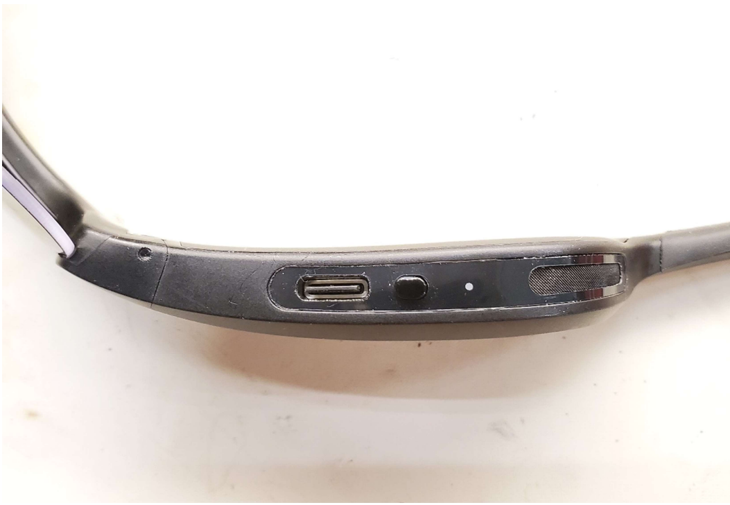
Right temple bottom with charging cable connection (USB-C), switch, and LED
