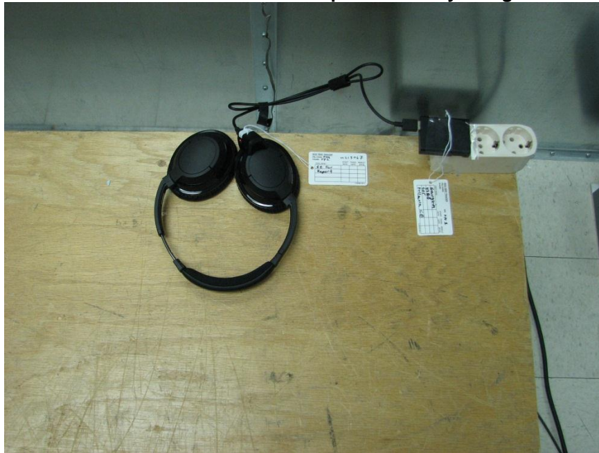
Conducted Emissions with optional battery charger
