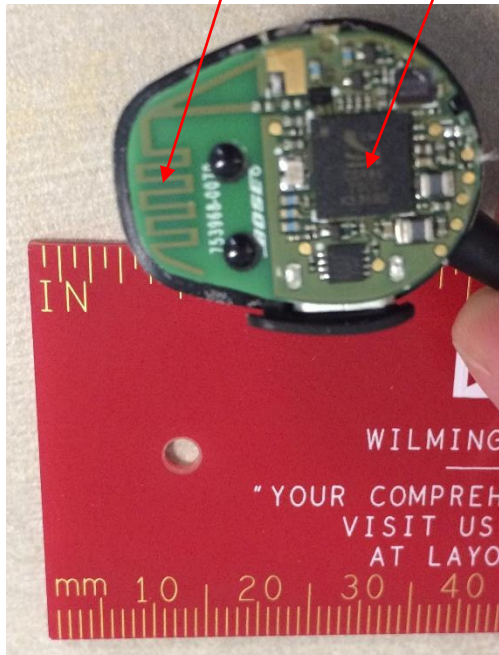
Right earbud, main PCB bottom side
