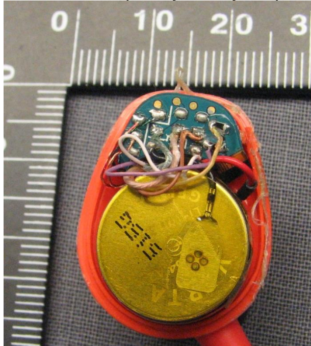
Left earbud (Battery, Battery PCB)
