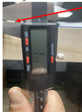
Supporting board thickness = ~1.6 mm
