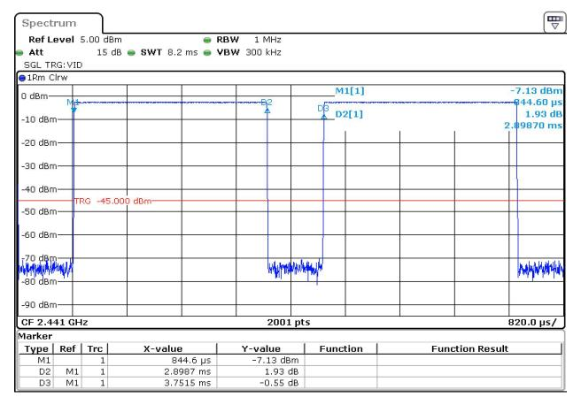
DH5 packets transmitting in test mode. Marker D2 = Time ON, Marker D3 = Period.
