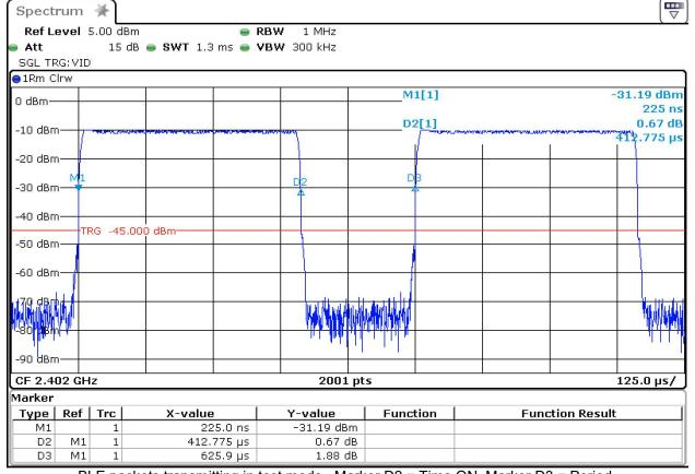
BLE packets transmitting in test mode. Marker D2 = Time ON, Marker D3 = Period.
