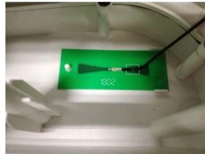
Antenna is secured on the product cabinet with adhesive
