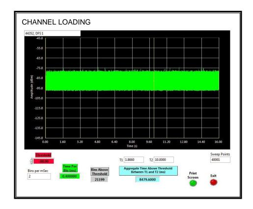
The level of traffic loading on the channel by the EUT is 84.796%.
