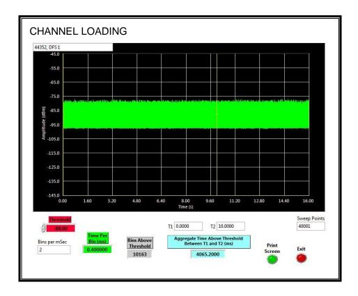
The level of traffic loading on the channel by the EUT is 40.652%.
