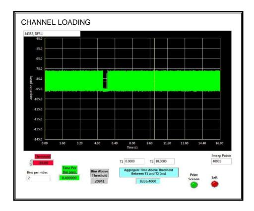
The level of traffic loading on the channel by the EUT is 83.364%.
