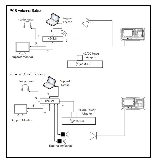
Note: Conducted setups were the same, except spectrum analyzer was connected directly to the antenna port.
