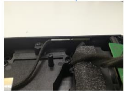
Antenna secured on EUT cabinet with adhesive
