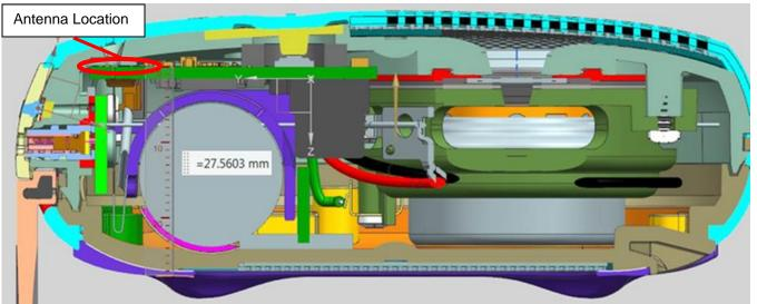
Measurement from the top side of the PCB where the PCB etch antenna is located. The distance is measured from the antenna to the bottom foot because that is the closest distance to a customer in a body worn condition if they were to use the included strap to attach the EUT to their belt. If it were not for the potential to attach to a belt this product would be a portable product and we would be applying for the more lenient MPE exemption instead of SAR exemption.
