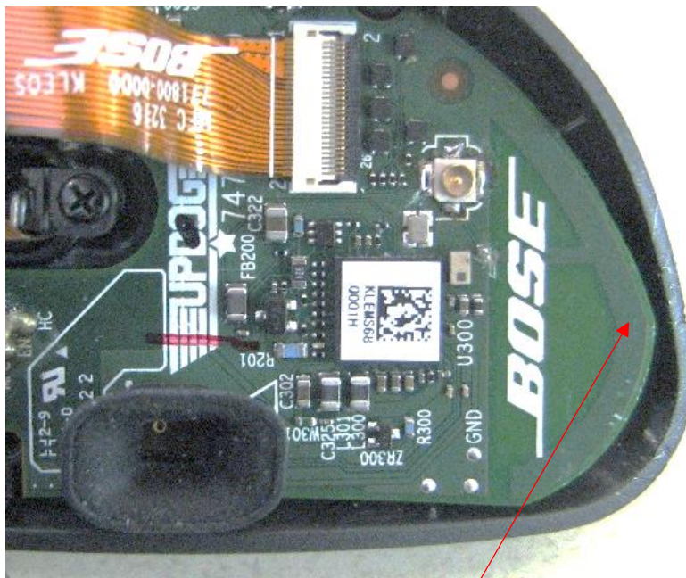
Inside view showing PCB etch antenna (Antenna gain is 1.84 dBi)
