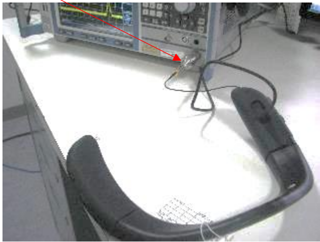
Setup with 2.4 GHz notch filter & 10 dB Pad
