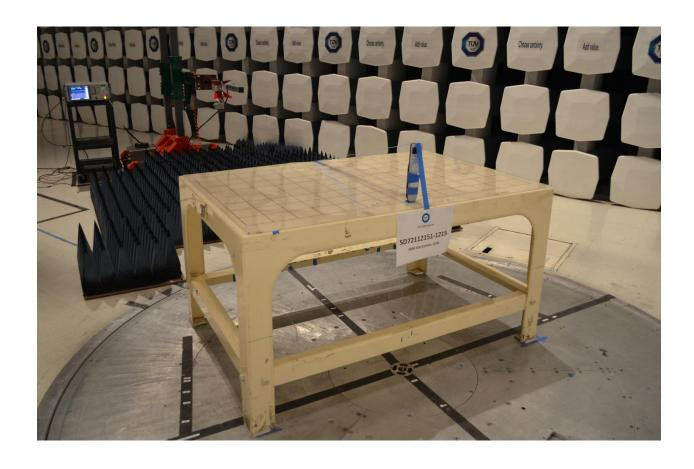
Radiated Emissions Test Setup (above 1GHz Back)
