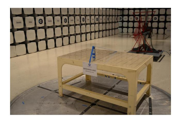
Radiated Emissions Test Setup (below 1GHz Back)
