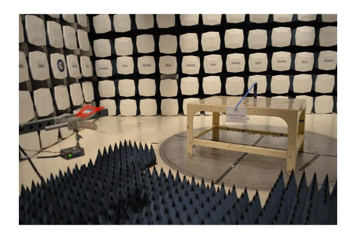
Radiated Emissions Test Setup (above 1GHz Front)
