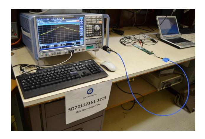
**Antenna Conducted Port Test Setup**
