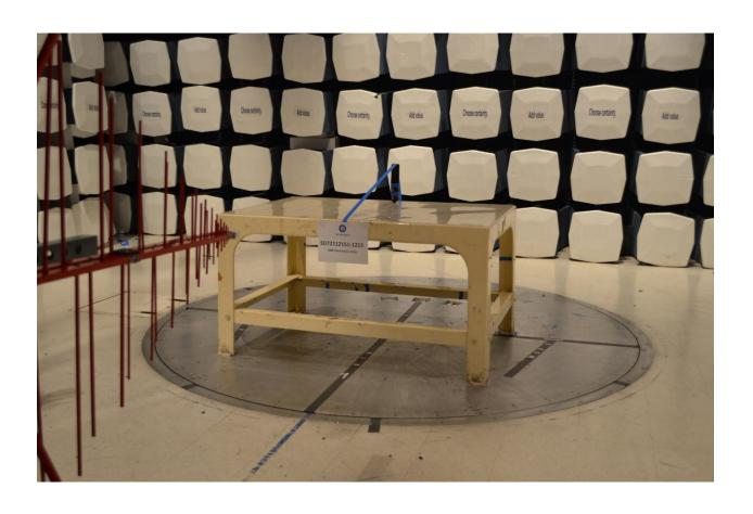
Radiated Emissions Test Setup (below 1GHz Front)
