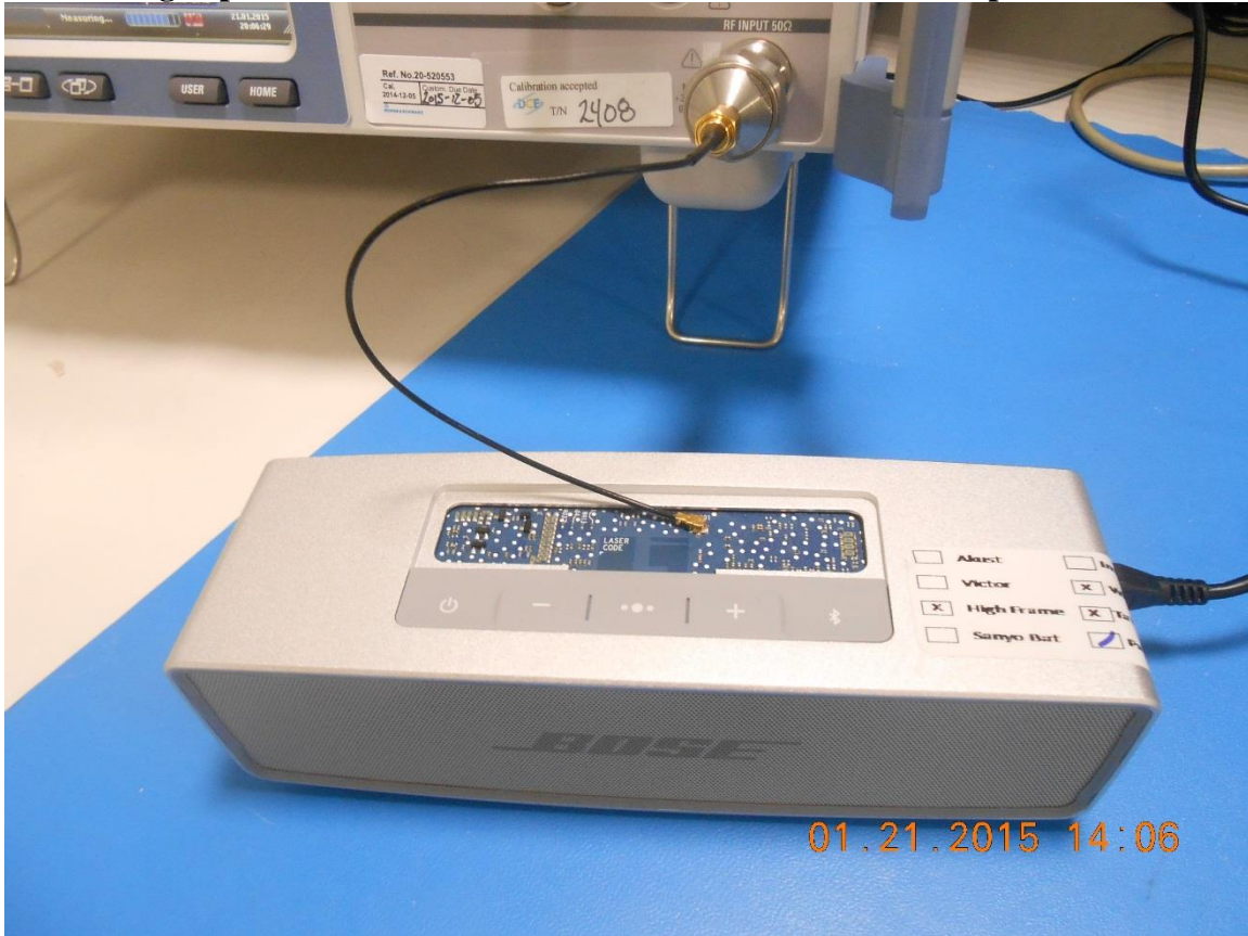
Staged photo of how transmitter conducted emissions were performed
