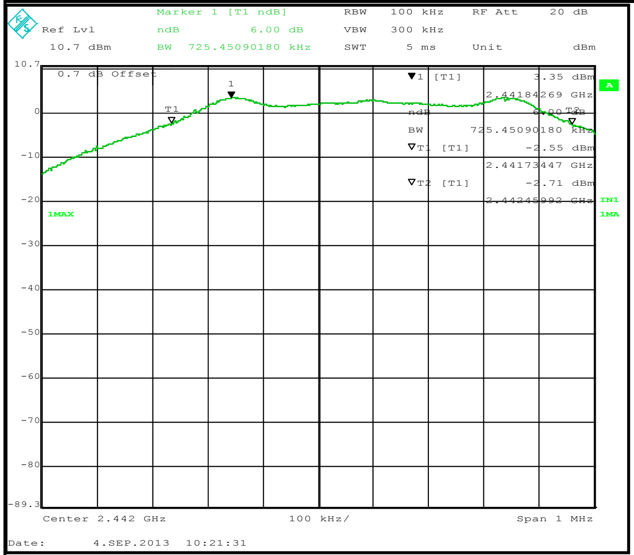
Representative plot showing 6 dB bandwidth measurement at 2.442 GHz
